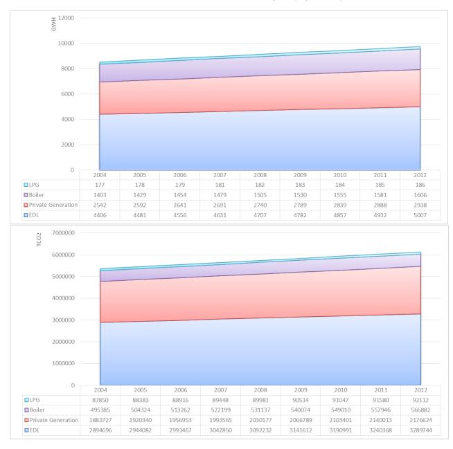
Figure 5-1 Energy Consumption (Top) and GHG Emissions (Bottom) in the C&I Sector (2004-2012)
